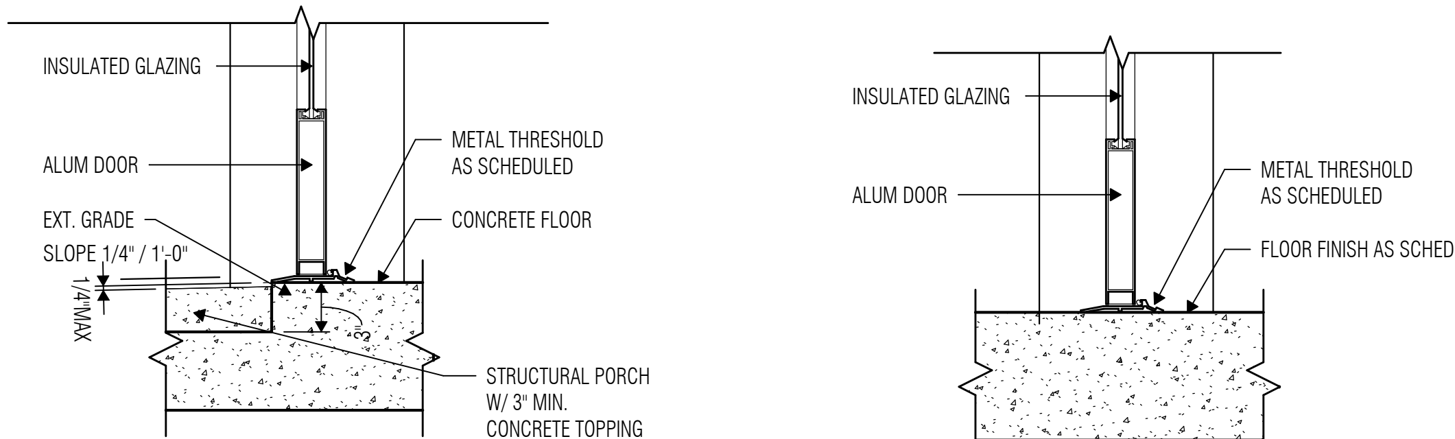
8 THRESHOLD DETAIL A EXT. DOOR SCALE: 1 1/2" = 1'-0" 9 THRESHOLD DETAIL A INT. DOOR SCALE: 1 1/2" = 1'-0"
